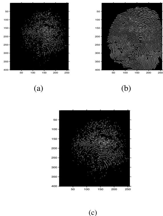
Fig 3: Output of edge detection of first fingerprints image (a) prewitt edge detection (b) canny edge detection (c) sobel edge detection
